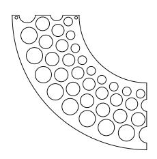
The main structure of the LAB.SP treeguard is in cold galvanised and polyester powder coated steel EN10111DD1, T. 50/10. The laser cutting process permits different kinds of decoration and so various patterns and designs are available. The TREEGUARD LAB.SP consists of four or two sections, each one
