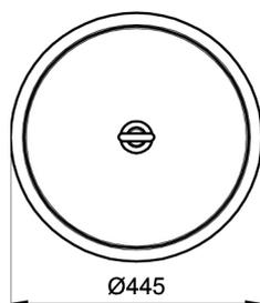
**Product:** Bollard with circular section model “MEL”, composed by two elements, a central band in between and an eyebolt for its handling or for a go-through chain.
