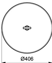
**Product:** Monolithic bollard with circular section model “TIP”, composed by a base and an eyebolt for its handling or for a go-through chain.
