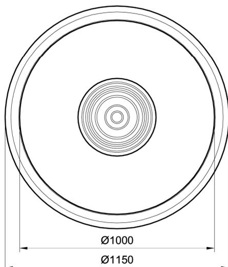
**Product:** Planter model “ESTATE”, composed by a planter and a base fitted with a **water reserve system** to guarantee the soil the proper humidity level, avoiding the dispersion of internal water, and with a **levelling system**, which allows compensation for the slope of the ground by up to a maximum of 4%.
